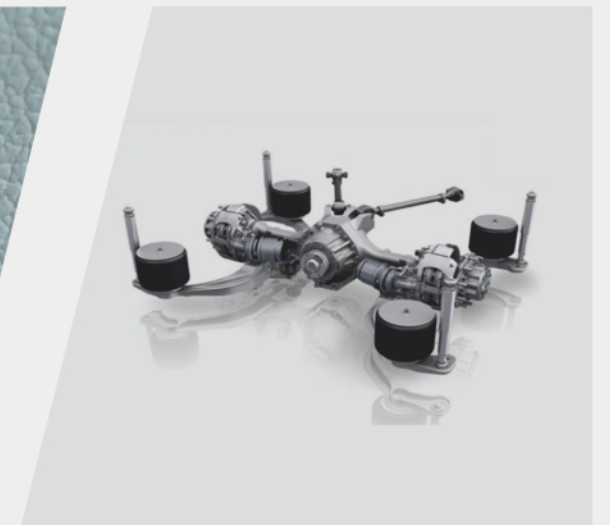
Airbag Suspension The front 2 and rear 4 airbags are effective in shock absorption, ensuring a steadier ride.
