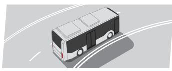
Maneuverability for easy drive Less than 8m of turning radius helps you navigate twists and turns.
